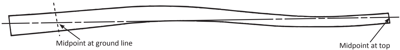
Diagram 3 — Measurement of short crook (three cases shown)
