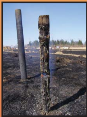
At right is a line of poles treated with fire retardant coating; in the background, smoke appears from an approaching wildfire. Above is a coated pole and an uncoated pole after a field test.
