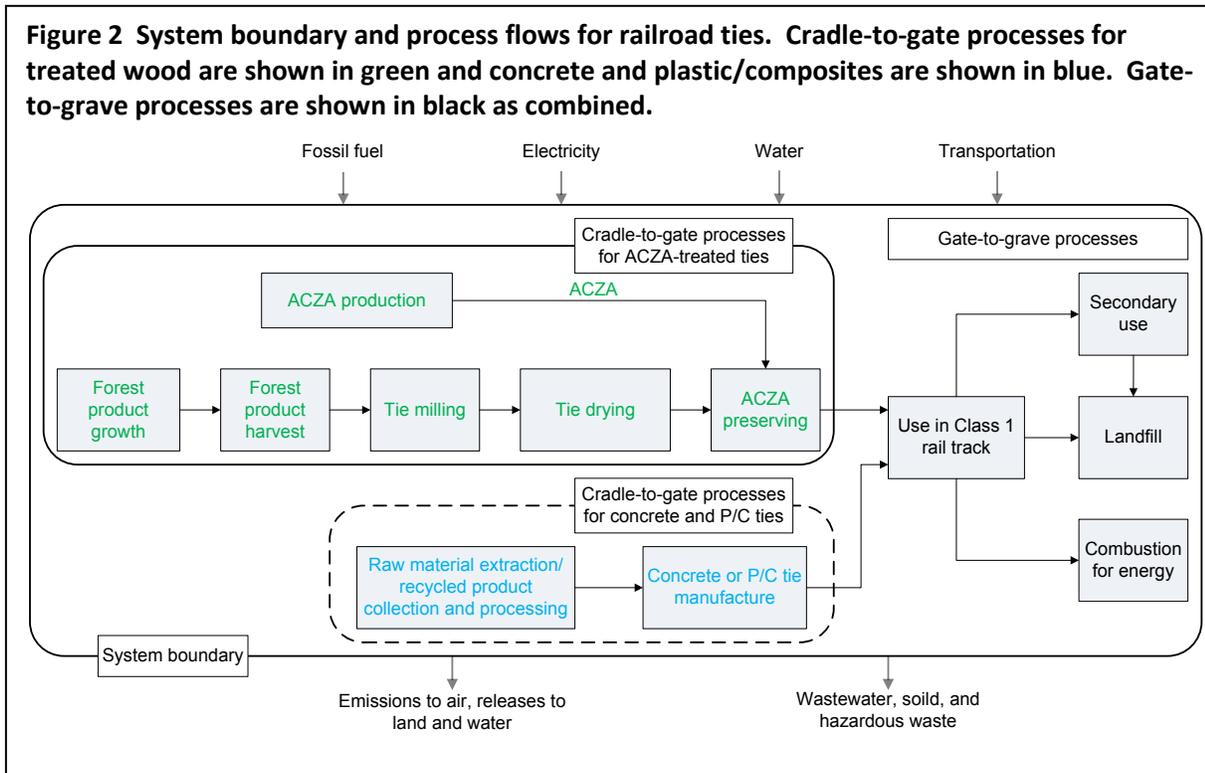
The length of time a railroad tie remains in service is dependent upon a number of factors. For this assessment ACZA-treated railroad ties were assumed to remain in service for 35 years. Concrete ties and plastic/composite ties are assumed to provide 40 years of service.
