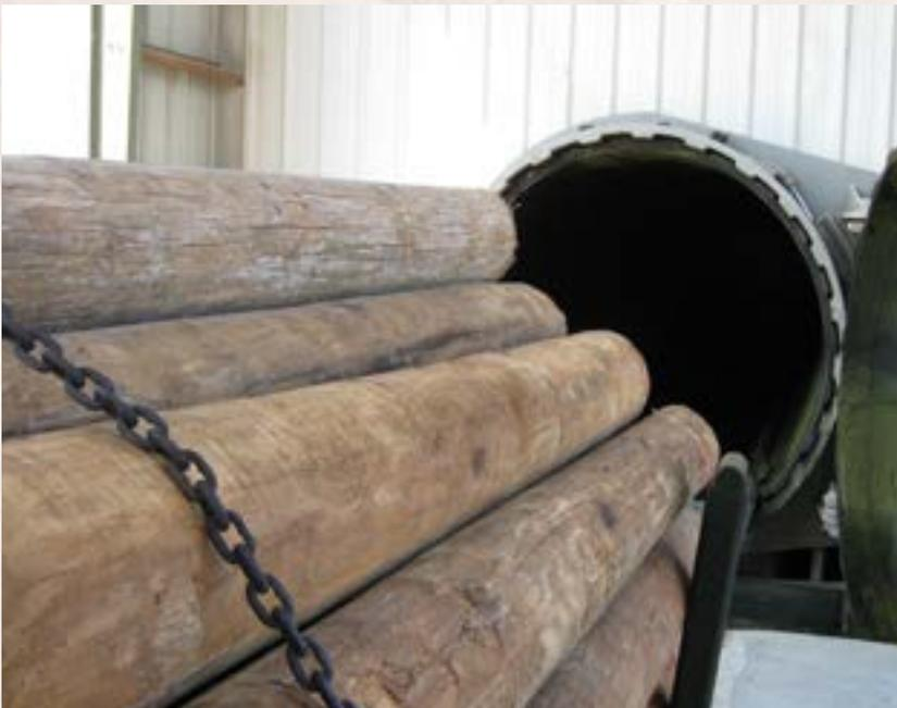
*Poles are moved into a treating cylinder where CCA is forced into wood under pressure. When treating is completed and CCA poles are pulled from the cylinder, approximately 80 percent of the preservative is "fixed" in the wood. Further fixation occurs soon thereafter, leaving the poles highly leach resistant.*
