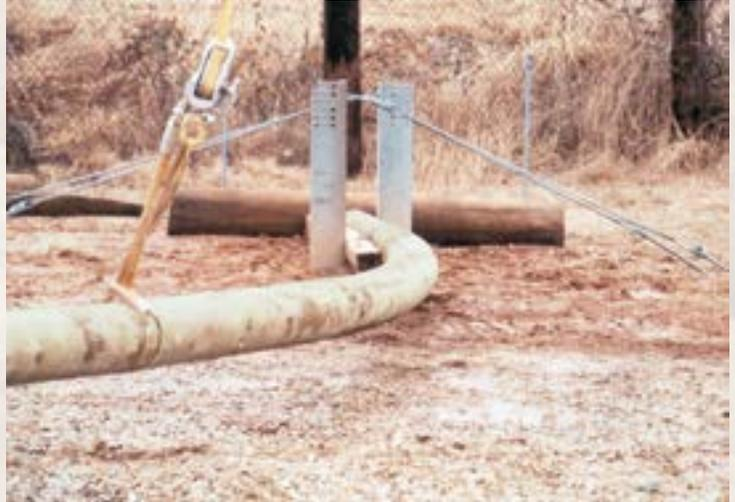
An eastern utility has subjected CCA poles to strength tests. All samples passed ANSI design criteria, some deflecting more than seven feet before breaking.
