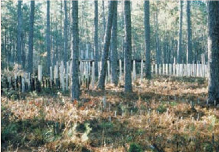
*Stakes treated with Wolmanac preservative and embedded in a test plot, such as the one pictured here, by the U.S. Forest Service in 1934 have shown no sign of failure from decay or insects. Untreated posts failed after just three years.*
