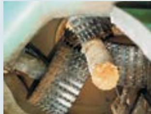
2. Pole-quality trees are processed to remove bark and the cambium layer, and to trim all branch stubs and overgrown knots. Waste removed during these steps is recycled as bedding or landscape chips, or is used as a fuel.
