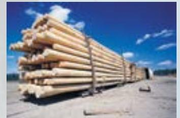
4. The poles are framed or cut to the specifications necessary for crossarms, before treatment. This ensures that the cut surfaces will receive adequate preservative treatment. Each pole is burn-branded or tagged so there is a permanent record of vital information about it for later reference.
