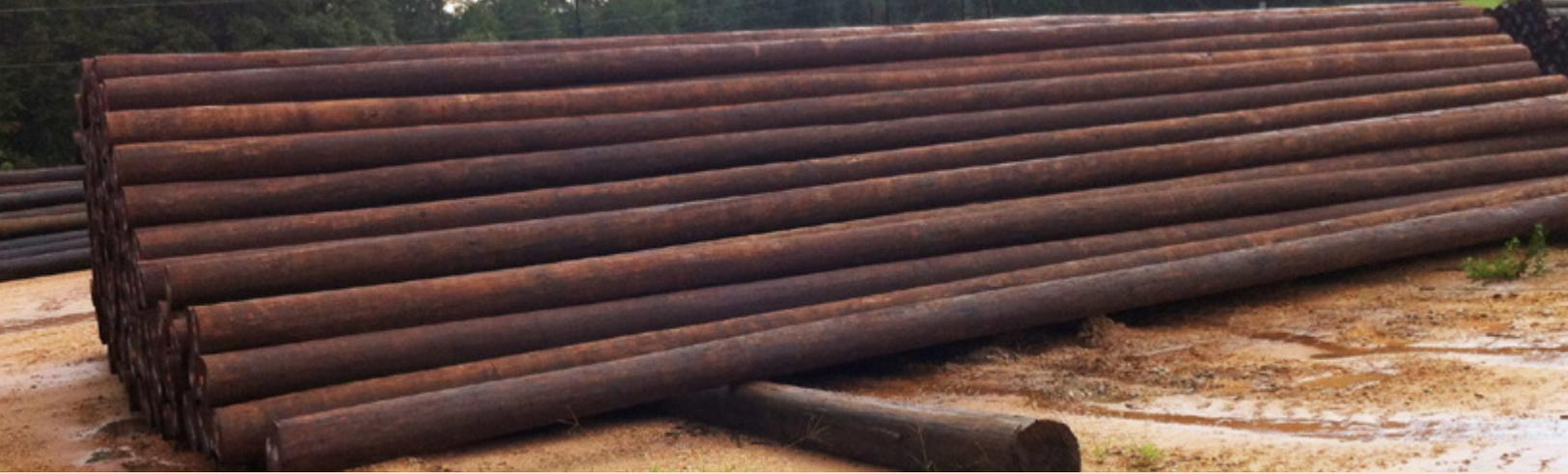
Following treatment with ACZA, the outer layer of ET® poles is treated with a refined hydrocarbon oil emulsion. This emulsion serves as a lubricant, making the pole easier to climb and to work on, without affecting the preservative properties of the ACZA treatment. The result is a number of practical features.
