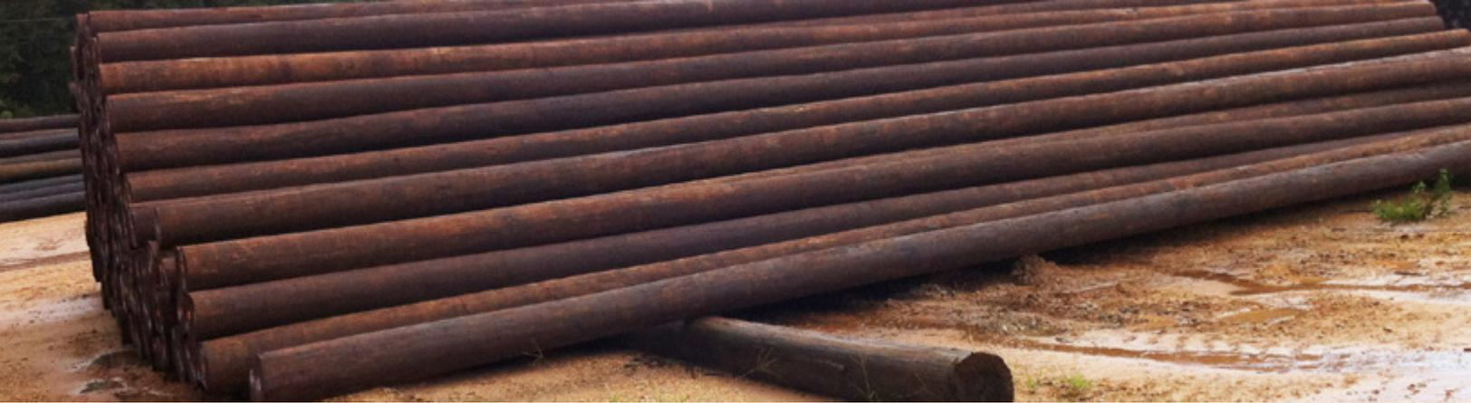
Following treatment with CCA, the outer layer of ET® poles is treated with a refined hydrocarbon oil emulsion. This emulsion serves as a lubricant, making the pole easier to climb and to work on, without affecting the preservative properties of the CCA treatment. The result is a number of practical features.
