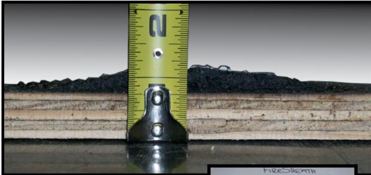
Above, a thin layer of FireSheath™ intumescent coating has swollen to a thickness that protects underlying wood. At right, with a burner held 7.75" away for 5 minutes, this coated plywood was affected in only a confined area.
