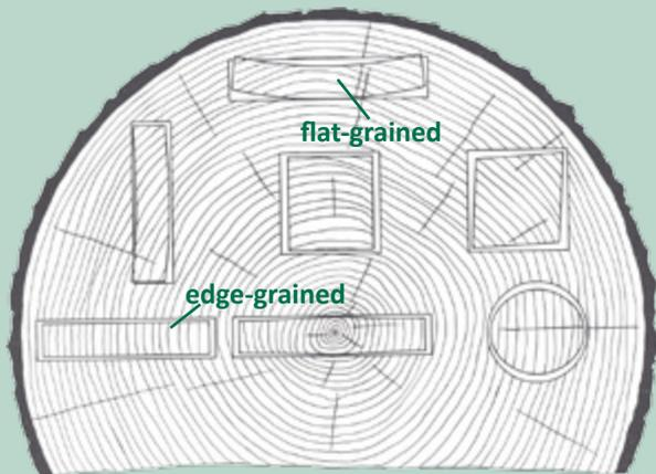
*This representation of a log shows how characteristic shrinkage of wood items depends on position in the cross-section. Radial shrinkage is about half as great as tangential. (Note: most logs are not this large, and posts and timbers usually come from the center.)*
