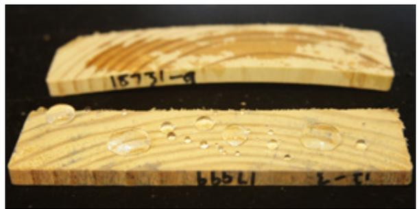
*This simple wafer test shows the effects of water on two sample pieces of wood. The front wafer, treated with Wolman® E Copper Azole with Lumbrella® Plus additive protects the wood by keeping water from penetrating, thus warping it. Wood without Lumbrella® Plus additive (back wafer) absorbs water, causing it to warp.*
