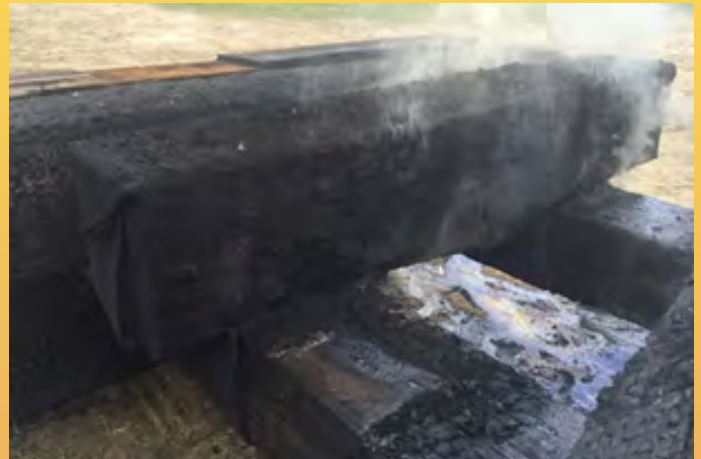
Wrapped ties cooling after fire; no visible signs of damage to ties wrapped with FireSheath® WFS Net™ mesh
