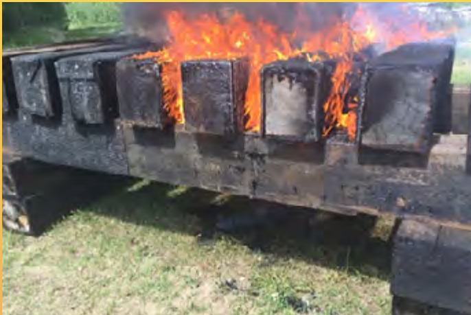
Unwrapped railroad ties fully engulfed in flames during test; wrapped ties not burning
