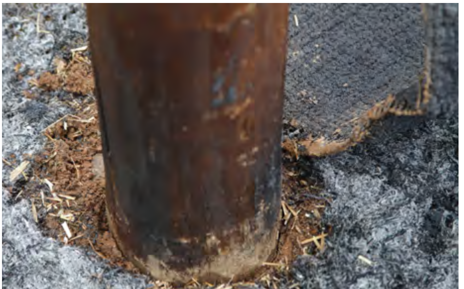
Post with FireSheath® WFS Net™ mesh removed after fire
