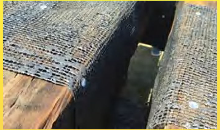
Railroad ties wrapped with FireSheath® WFS Net™ mesh before testing
